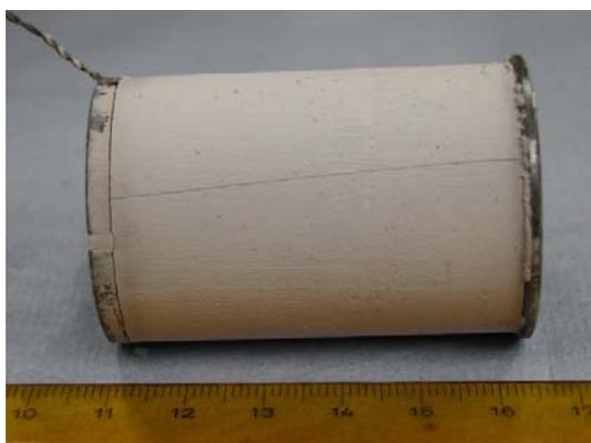
Fig.4.2.1a: ceramic-filled pick-up coil after curing process
