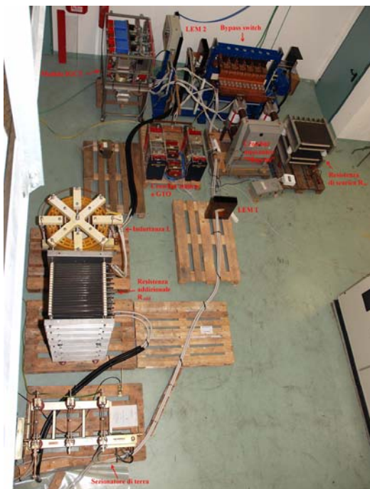
Fig.7.1.1: Development of a hybrid dc circuit breaker (10kA, 1kV) – test arrangement
