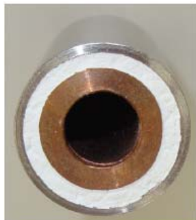
Fig.7.2.2: Picture of MIC with sheath made of SS316L
