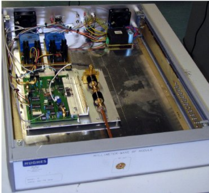
Fig.6.11.2: A complete microwave source unit (V band) using the new IMPATT driver.
