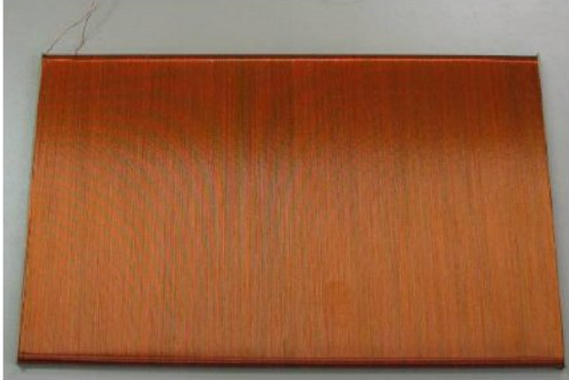
Fig.3.4.1: Prototypes of tangential coils manufactured in the framework of F4E-GRT-012 (overall dimension: 200x159x9 mm; nominal effective area :2 m 2 )
