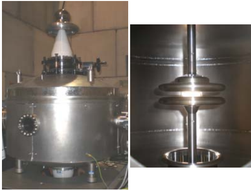
Fig. 3.3.1: 300 kV tank and \text{AlO}_2 feedthrough and the internal electrodes
