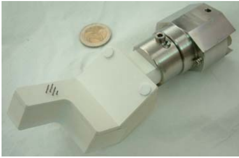
Fig.4.10.1: Picture of the probe head installed and commissioned in the TJ-II experiment
