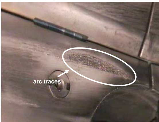
Fig. 1: image of W deposited tiles after about 450 plasma discharges
