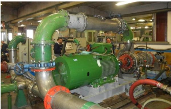
*Fig. 4.6: Tests of cooling plant pumps at manufacturer premises (Garbarino Spa, Acqui Terme, Italy, the 9/10/2014)*
