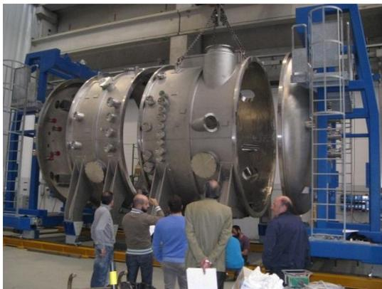
*Fig. 4.10: SPIDER VV during assembly at Zanon for factory tests*
