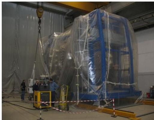
*Fig. 4.11: SPIDER Vacuum Vessel during global He leak tests (vacuum inside, He inside plastic bag)*
