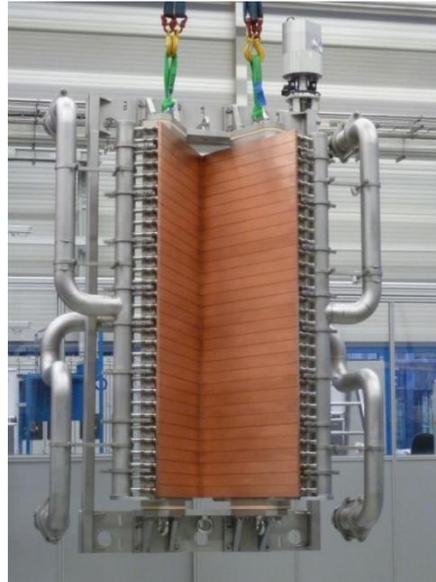
Fig. 4.20: Rear and front views of the SPIDER Beam Dump assembled at the Supplier's factory (PVA TePla)
