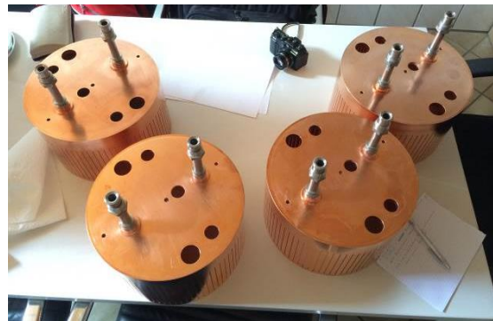
Fig. 2.1.20: SPIDER Faraday Shields Lateral Walls manufactured and tested by Galvano-T
