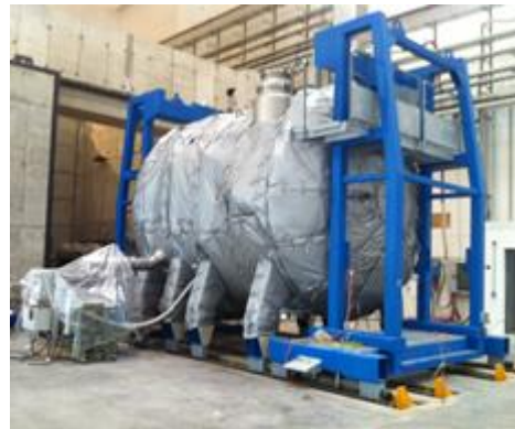
Fig. 2.1.15 :SPIDER VV during baking
