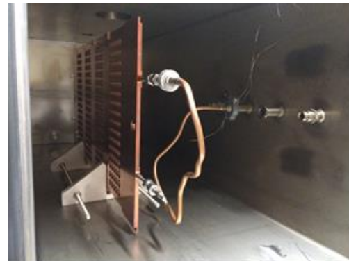
Fig. 2.1.18: In vacuum He pressure and leak tests of the cooling circuit of Plasma Grid segment
