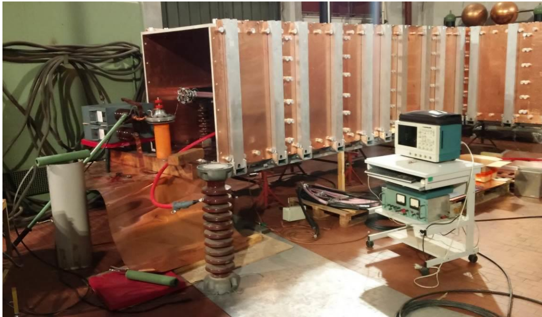
Fig. 2.1.27: Factory tests of the SPIDER Transmission Line
