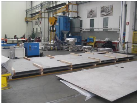
Delivery of SS sheets for vessel walls
