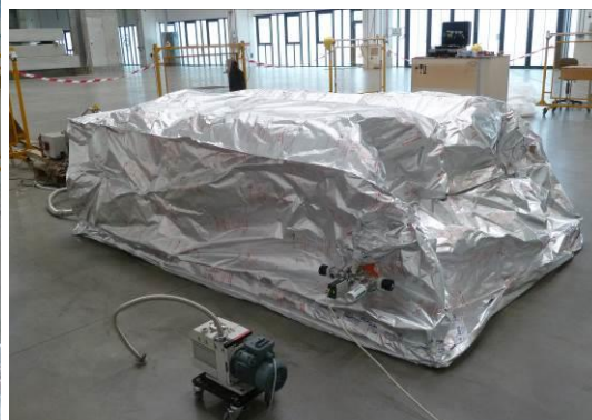
leak test: Internal cooling circuits evacuated and He atmosphere around the component
