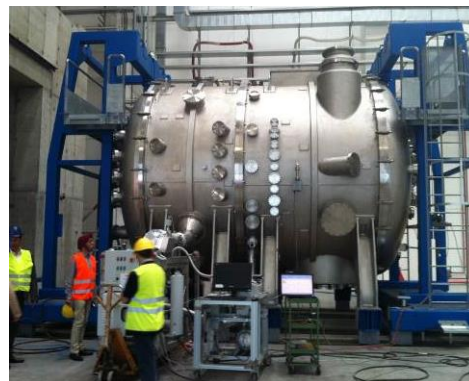
Fig. 2.1.16: SPIDER VV during vacuum tests on-site
