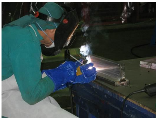
Welding qualification process
