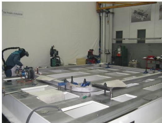
Manufacturing of a first large connection flange for the Vessel.
