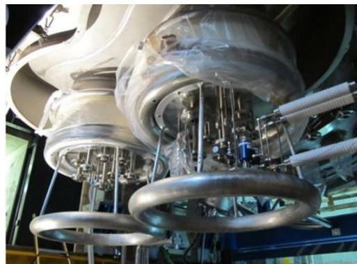
**Fig. 2.1.1** The finally assembled hydraulic bushings on the bottom side of SPIDER Vacuum Vessel
