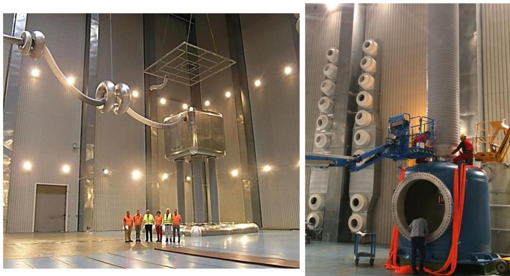
**Fig. 2.1.41 (left) HVD1 mock-up inside HSP laboratory for Insulation tests, (right) HVBA during assembly for pressure tests**
