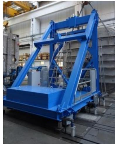
**Fig. 2.1.29** Tests of Rear Lid Handling System at supplier's workshop
