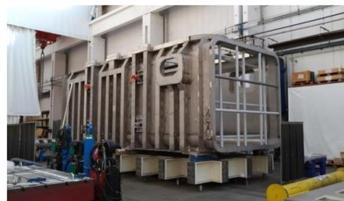
**Fig. 2.1.31** Pictures of the Beam Source Vessel (metrology works) and Beam Line Vessels at supplier's workshop
