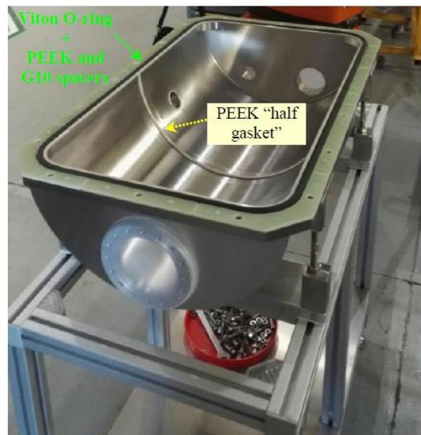
**Fig. 3.1.13 Mock-up realized to test VTSS vacuum-tight electrical-insulated crossed joints**
