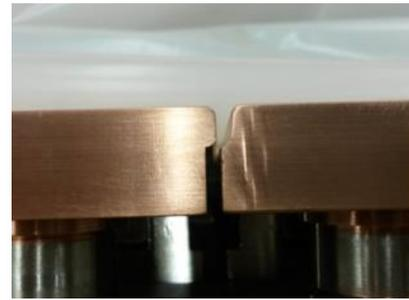
**Fig. 2.1.11 Detail of a typical shinethrough between adjacent hypervapotron elements of SPIDER Beam Dump**
