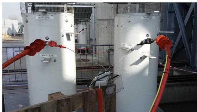
**Fig. 2.34 Setup of the line to line voltage measurement at the ringing filter connection.**
