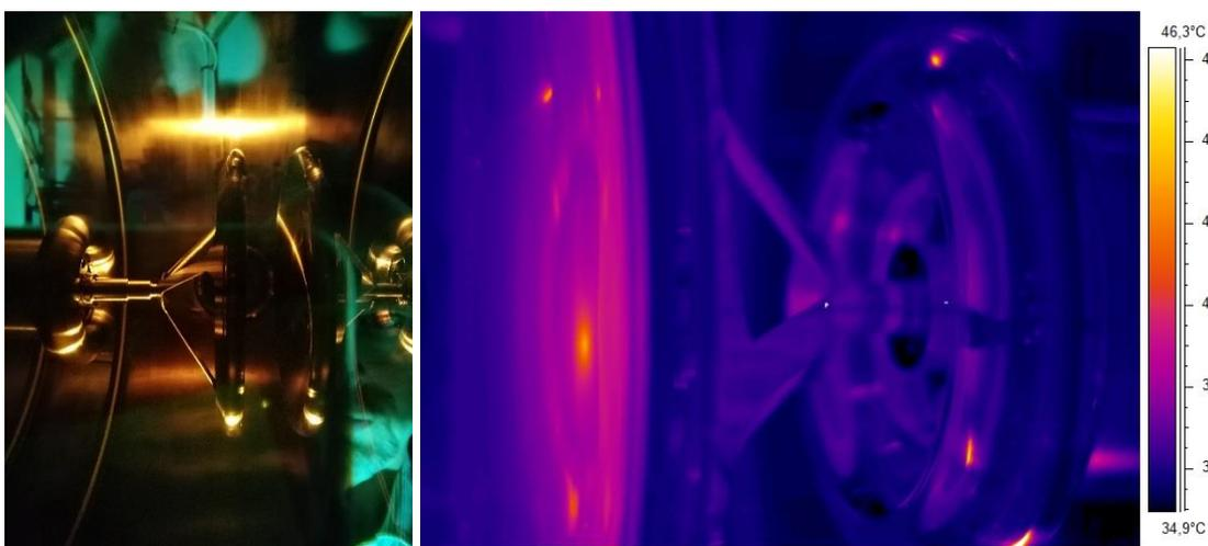
**Fig. 2.54 Picture of the concave electrodes taken during the assembly (left). Hot spot on the centre of the concave anode during the HV conditioning (right) in presence of microdischarges**
