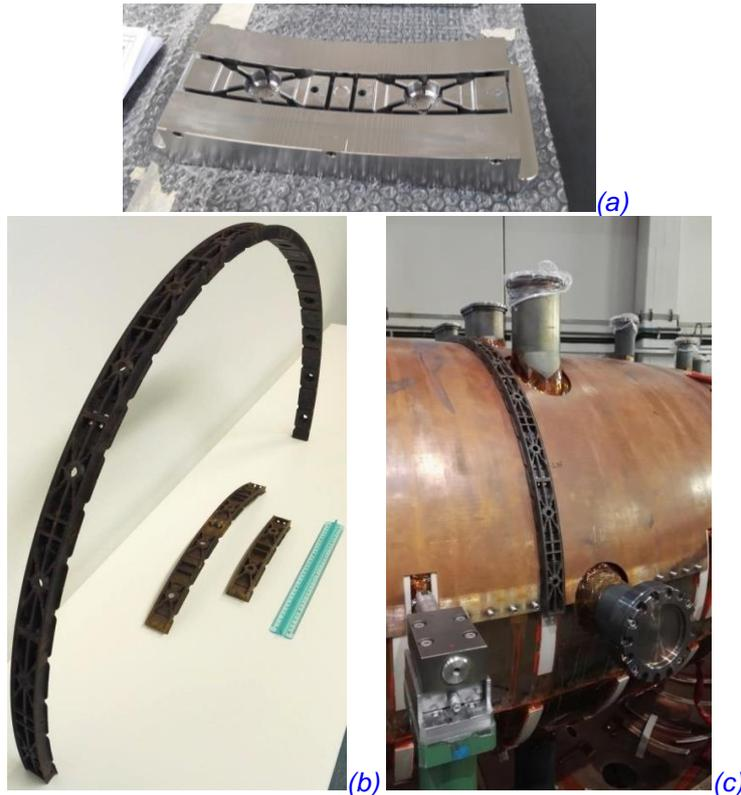
**Fig. 3.5 Manufacture of Torlon rings prototypes: (a) injection mould; (b) ring sectors prototypes; (c) assembly test on the PSS**
