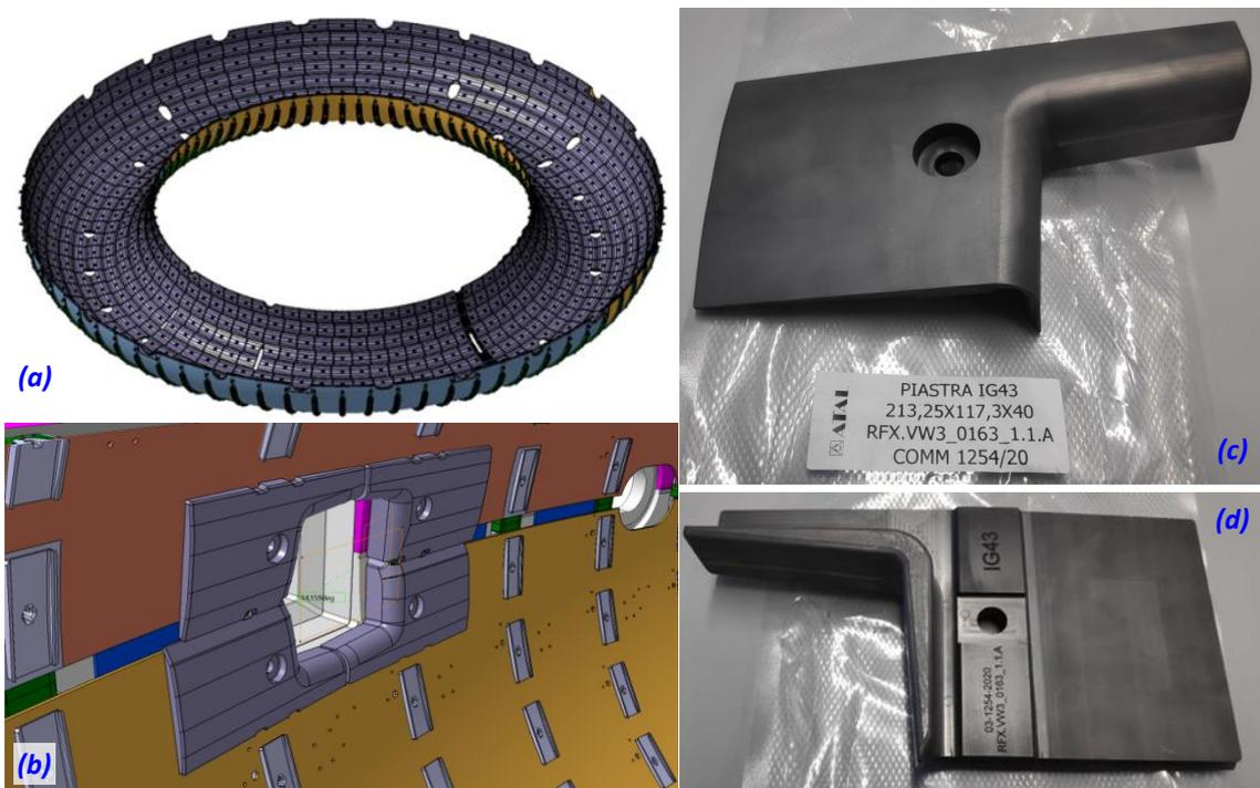
**Fig. 3.9 (a) CAD model of the entire first wall protecting the bottom part of the PSS; (b) detail of tiles at equatorial access of the VTSS; (c) + (d) graphite tile prototypes**
