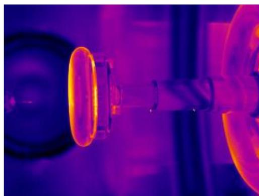
**Fig. 2.52 Infra-Red picture of the Needle-plane test. Electron backscattering can cause more than one hot spot on the anodic surface**
