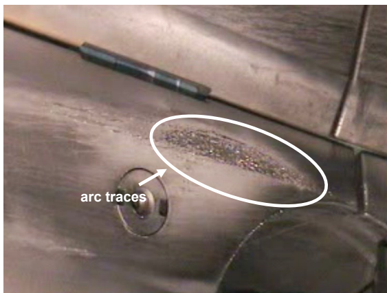
Fig. 1: image of W deposited tiles after about 450 plasma discharges
